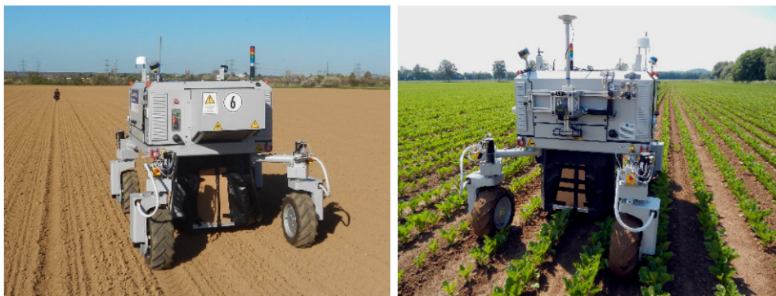
Figura 8. Robô BoniRob (CHEBROLU et al., 2017).
