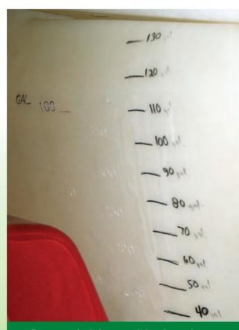
A flow meter check determined that the markings on this tank are all off by 10 gallons. Make sure the flow meter is correct by calibrating it according to the manufacturer's instructions.
