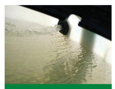
Polyethylene (poly) tanks may employ pressurized bypass agitation to maintain a uniform mixture. In some cases, valves can be installed to better direct the incoming water at the bottom of the tank.
