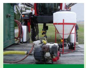
With today's sophisticated equipment, electronic flow meters can be a great asset when filling sprayers. In this case, the digital readout is mounted in a position that makes it easy to read during the filling process.
