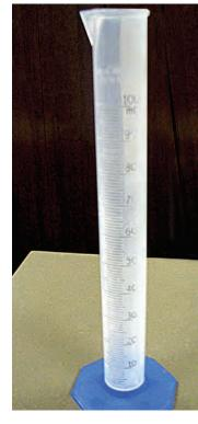
(Left and far left) Use graduated glass or plastic cylinders that allow for precise measurements. (Left) The units on this cylinder are 1 milliliter apart. (Below left) It is impossible to accurately measure 236 milliliters with this glass beaker below, since there is no mark for this amount.
