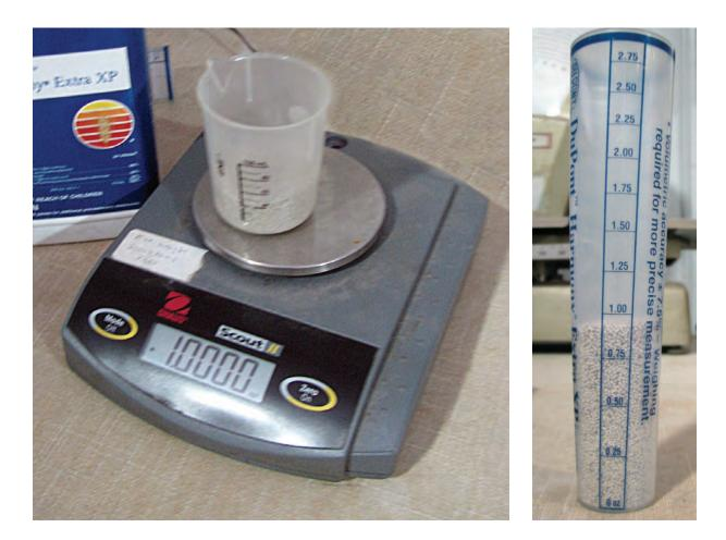
Select a scale that allows you to tare (zero) out the weight of the container (a plastic cup in the photo above left) in which the dry materials are placed. In this example, the plastic container was weighed. With the push of the "tare" or zero button, the weight reads zero. By adding the material after you tare the device, you will get a reading that does not include the weight of the container.
