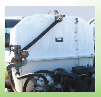
GAL. Measuring the tank 4 F.I to ensure that its markings are correct 160 is an easy step that can lead to more precise applications. Notice the difference 150 . in where the 30-gallon mark is and the actual 140 measurement taken with a flow meter. Make sure the tank 130 is level when 130 remarking. 120 -
