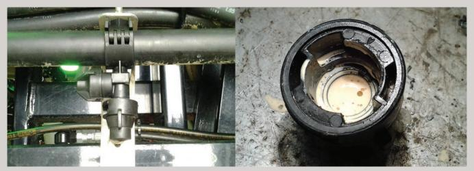
The right photo shows herbicide residue that was left in a drop nozzle from a previous use.
