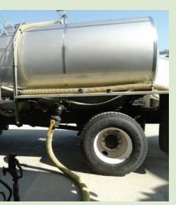
**Hoses used to fill tanks with water** can be sources of herbicide contamination. Typically, permanently mounted hoses move herbicide from bulk tanks and water. Most often, you can color-code these hoses: a yellow hose might indicate products used on corn, while a black hose might carry products used on soybeans. Color-coding hoses ensures that any residues remaining in the lines are applied only to a nonsensitive crop.
