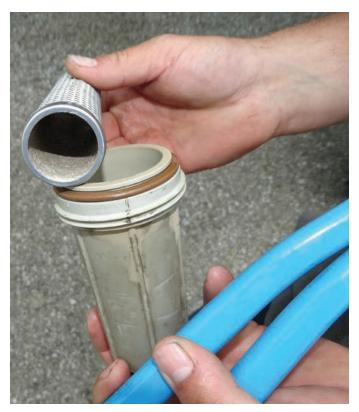
The buildup in a screen may not always contain active herbicide. This image shows a screen with clay particles from formulations and CaSO<sub>4</sub> from adding AMS for hard water.
