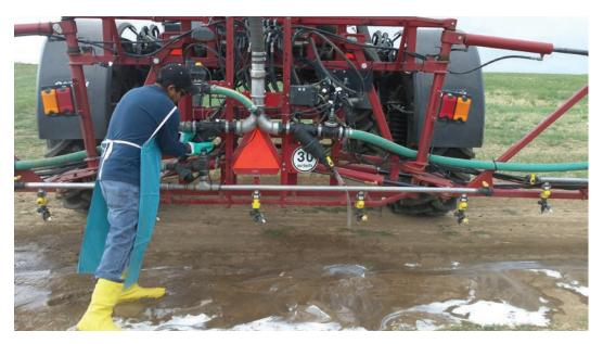
This sprayer has two screens at the rear for each side of the boom. Note that the applicator is wearing personal protective equipment.
