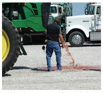
A red dye in this spray mixture mimicked an herbicide. This demonstrates why you need to clean out the front load. If not purged, any chemical that remains will be pushed back into the tank when you pump the next load into the sprayer.
