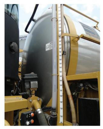
Replace sight gauges several times during the season. It's only a few bucks, but replacing these gauges can eliminate residues that can embed in the plastic. It's been suggested that unhooking the top and pulling the hose down will allow any trapped herbicides to exit.
