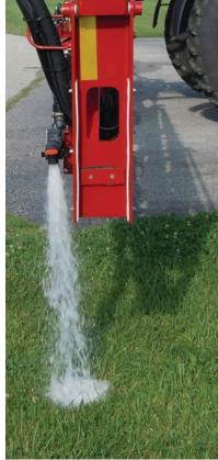
Attaching a quarter-turn valve at the end of each boom section allows for easy flushing.
