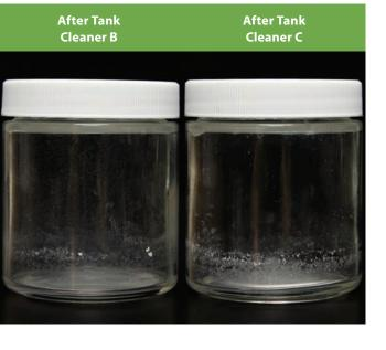
Ammonia has difficulty removing dried-on herbicide residues. It is important to use high-quality tank cleaners that contain surfactants and other materials that can break down dried residues found in sprayer systems.
