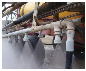
How much water you use during the first rinse is based on experience. In all cases, water coming out of the nozzles needs to pass the eye test. In other words, water should be clear without any evidence of a tint or sheen (top). Be sure to open the end nozzle during the first flush. Continue to add water to the tank until the water exiting the nozzles is clear.
