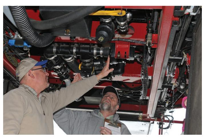
Sprayers have complicated interconnections of hoses, filters, and valves to control flow and pressure. A standard operating procedure and cleanout checklist will ensure that you omit no step.
