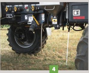
Some application equipment may have a ball valve at the end of the screen nearest the pump (photographs 1 and 2). The ball valve allows the screen to be easily flushed when you open the valve. While opening the valve can remove a significant amount of residue from the inside of the filter, you should never just open the valve and skip manually cleaning the screen (photographs 3 and 4). The only way to thoroughly clean a screen is to remove it and to use a brush with tank cleaner and hot water.
