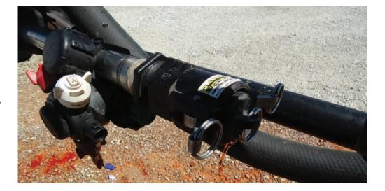
This end cap has been modified with a quick coupler to allow for easy removal and cleanout. Make sure to use a plastic tie on the lock rings to secure the coupler.
