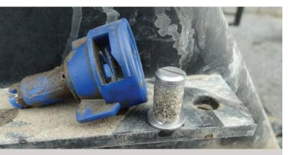
Fewer applicators are using screens at the nozzle tips than they once did, because it takes too much time to clean that many screens. There are 96 nozzles on a 120-foot boom. Most manufacturers of new sprayers rely on the other screens to remove debris before it gets to the tips. However, for those other screens to be effective, they must be 50- or 100-mesh to do the job. Check the manufacturer's instructions — they suggest screen sizes.
