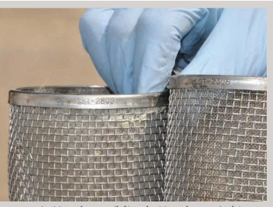
An 80-mesh screen (left) and a 30-mesh screen (right).
