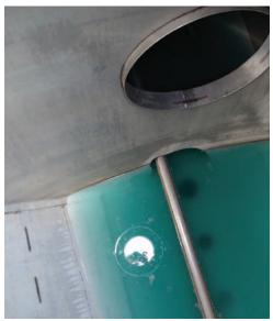
Side wall cleaners (left) and sparger/agitation bar (right).
