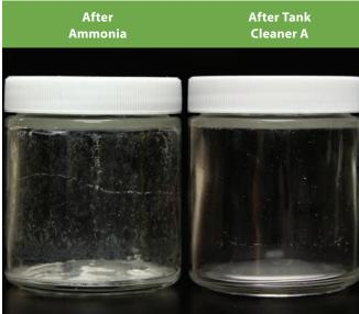
Oil sludge can be difficult to remove as is shown with using only ammonia. There are also differences in a tank cleaners ability to remove oil residues.
