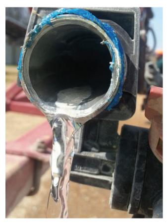
Considerable herbicide residue can build up on the inside of the end cap or in the boom. See page 37 for end caps that are easier to remove and clean.
