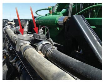
An often-overlooked part of cleaning a sprayer is the system of hoses that move liquid through the flow meters (meters marked with red arrows).
