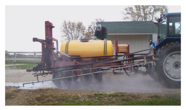
Make sure to open the front and side loading valves (including the plumbing) to the injectors a few times for a few seconds to allow water to circulate through the pumping system. This will push the remaining spray mixture through the booms and nozzles. Spray this mixture over the last crop until the pump loses its prime again — this allows the sprayer to discharge most of the spray mixture.
