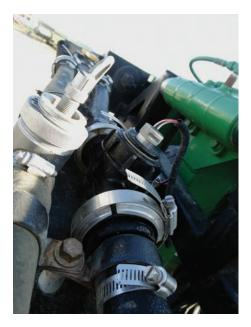
Some sprayers are equipped with dual flow meters for high-and low-flow rates. If you do not use the second flow meter, the herbicide may get trapped on the outlet side of the valve. If you do not flush the inlet after use, it is possible that the herbicide will sit in that section until you open the valve.
