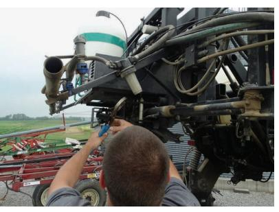
Always wear gloves and eye protection when you work around pressurized water or air while handling screens. The screens may contain concentrated product that has not dissolved.
