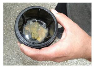
The screen in this water tank shows a buildup of algae (above) and rust (below).
