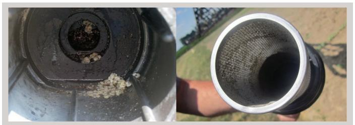
Materials accumulated in the filter between the tank and pump (left). The screen associated with this filter shows debris captured by the screen (right).
