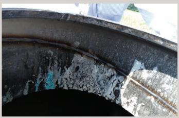
Some tank openings have locations that the side wall cleaner and agitation device cannot fully reach (left). In this example, a piece of metal runs around the rim of the tank opening where residues have built up (right). The only way to remove this residue is with a hose or high-pressure sprayer.
