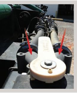
Notice the flow then comes together at a Y juncture (red arrows). Flow from one side of the Y can actually back up into the other. Unless you run clean water in each side, the remaining herbicide can become a contaminant.
