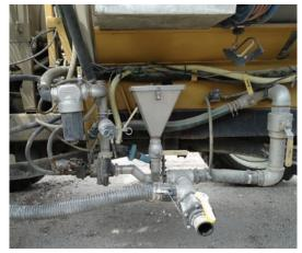
When circulating the tank cleaner through the sprayer system, make sure to open the valves to allow the cleaning solution to move into the inductor hoses. Some applicators add a small amount of tank cleaner directly to the inductor as an extra precaution.
