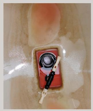
Some tank designs do not allow complete drainage. (Left) In this case, there is liquid contained below the drain opening that the pump will not be able to pull through the system. Other tank designs allow for liquids to completely drain out of the sump (right). The first 30 to 50 gallons of clean water will remove much of the tank mixture left in the sump area and in the hoses and booms.
